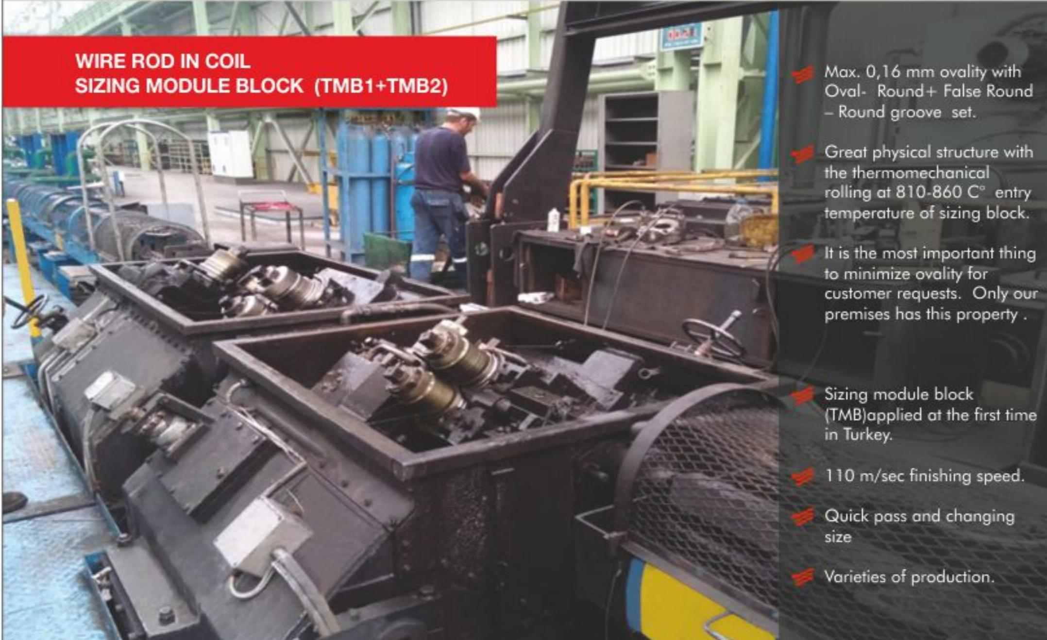
A large industrial machine, specifically a wire rod sizing module block, is shown in a factory setting. The machine has a complex metal frame with various mechanical components, hydraulic systems, and control panels. A worker is visible in the background, operating the machinery. The overall environment is a typical industrial manufacturing facility.
