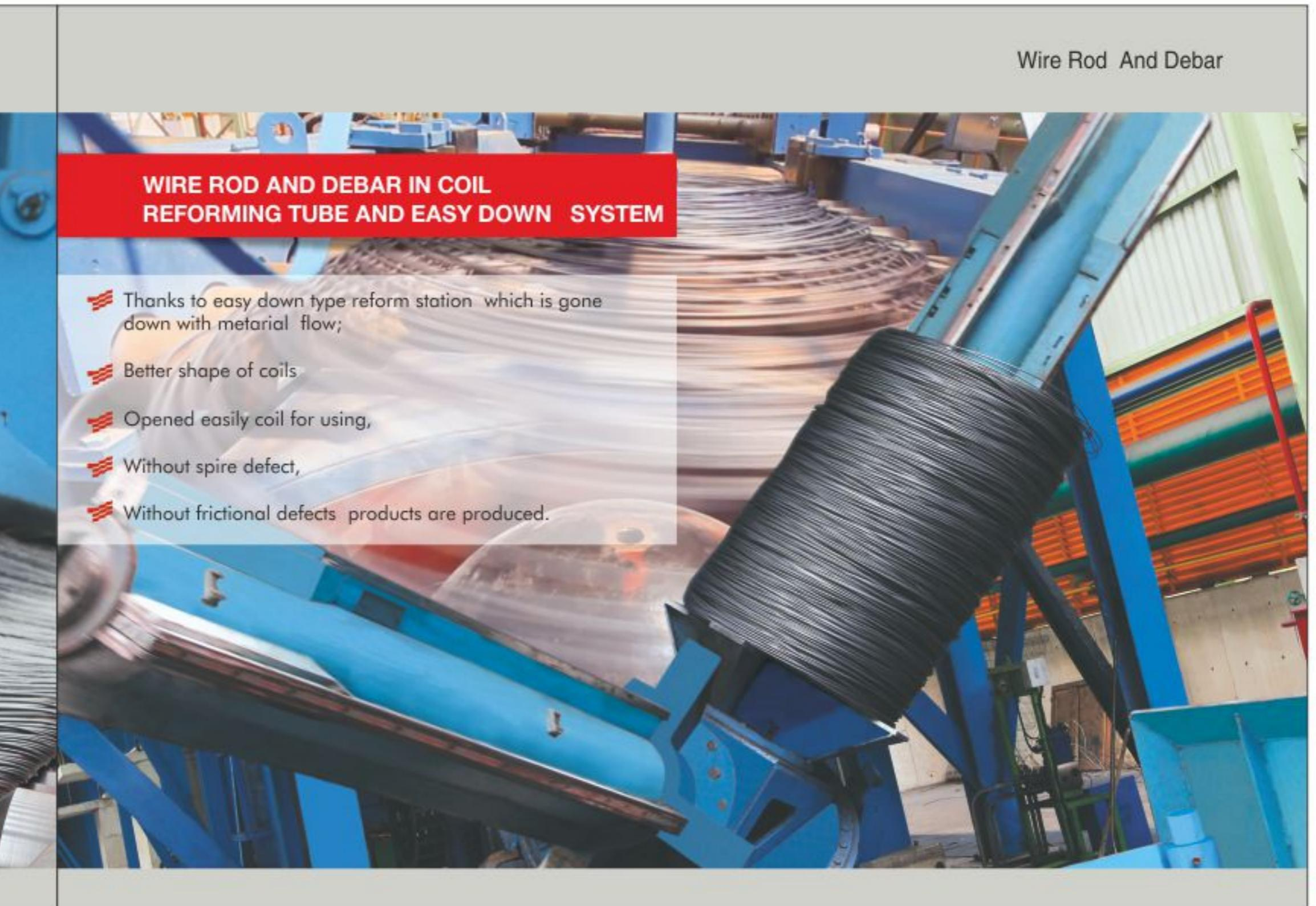
A close-up photograph of a wire rod and debar coil being processed. The coil is being fed into a blue-colored reforming tube. The tube has a curved section where the coil is being shaped. The background shows more of the industrial machinery and equipment.
