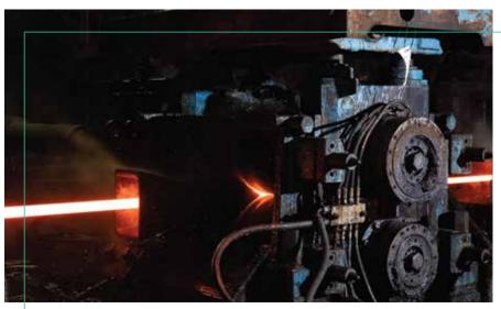
Surface defects are removed by descaling of four surfaces before rolling in all qualities.
